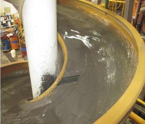
Figure 1: MG-12 spiral technology enables cut-off recovery rates to drop from 38 to 20 micron.
