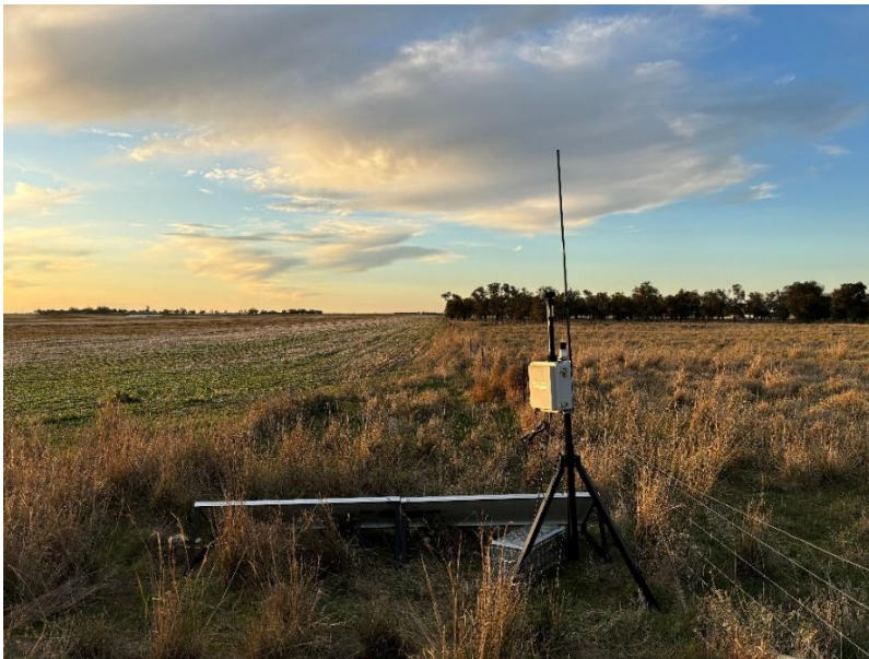
Dust monitoring station established on proposed mine site
