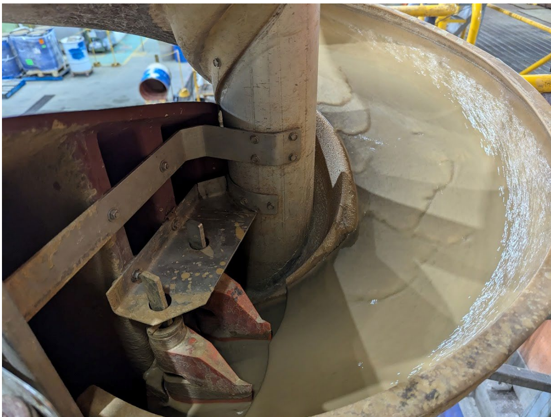
Figure 1. Gravity concentration of ore using a rougher spiral, part of the equipment test work conducted by Mineral Technologies, October 2024.
